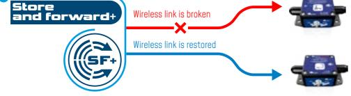
WIFI network is disrupted, all the measurements are recorded on the onboard datalogger
