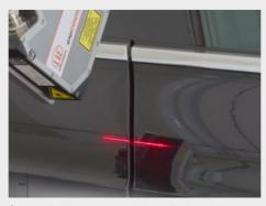
Gap and flushness measurement on bodywork parts
