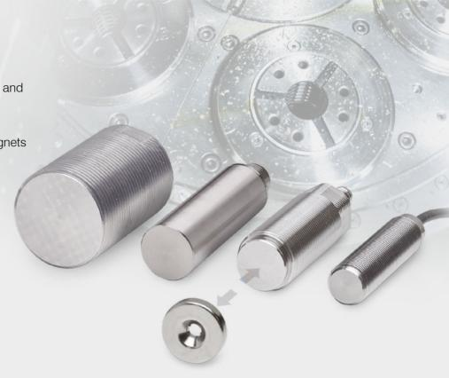
mainSENSOR distance sensors use an innovative measuring principle, which combines the advantages of both inductive and magnetic sensors. Measuring the distance to a magnet which is attached to the measuring object, the sensor outputs a continuous, linear output signal. By using magnets of different strengths, measuring ranges between 20 mm and 55 mm can be achieved. In order to adapt the measuring range, you only have to change the magnet.
