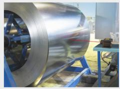
Acquisition of coil diameters
