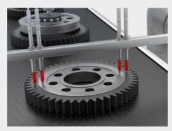
Checking the offset of gears
