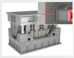
Monitoring the metal sheet infeed during pressing
