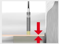
Monitoring the oil gap of drive shafts
