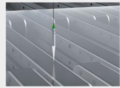
Thickness measurement of flat glass
