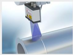
Scan of components before laser cladding
