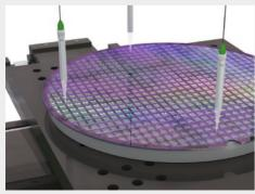
Inspection of wafer tilt angle
