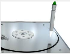
Inspecting the axial runout of hard drives
