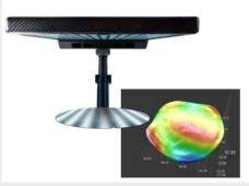
3D shape measurement of wafers
