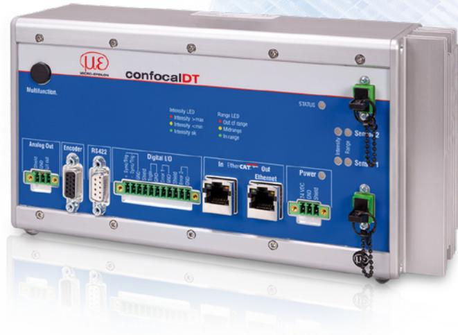
The confocalDT 2465 and 2466 controllers enable fast, high-precision distance and thickness measurements up to 30 kHz. They are available as a single- or dual-channel variant. In addition, the MP models measure the thickness of up to 5 transparent layers at once. The controllers are characterized by high luminous intensity which enables very fast and reliable measurements even on dark surfaces.
