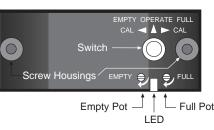
the sensor while calibrating because this will cause a false reading. Using a small nonmetallic screwdriver or alignment tool, turn trimpot Full until the LED just lights, and no farther. Note the position. Now turn the trimpot back until the LED turns off. The ideal setting for the trimpot is midway between these on and off points.
