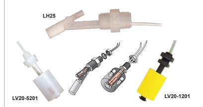
Offered in vertical and horizontal configurations, the general purpose mini-float level switches provide reliable liquid level detection of clean water and chemical solutions with a 15VA or 30VA reed switch output. Media examples include water and sulfuric acid. The polypropylene or PVDF liquid level sensors are mounted vertically inside the tank or horizontally through the tank wall as a high level alarm or low level alarm.
